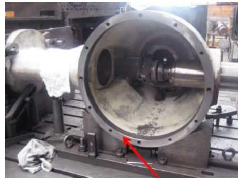
Img. Nr. 12: Line boring and skimming of joint surface.
